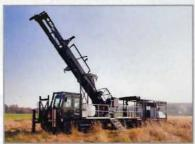
At MINExpo Boart Longyear will give attendees a first-hand impression of the recently released LS600 sonic rig. With advanced sonic-drill technology featuring patented designs, the LS600 delivers continuous, undisturbed core samples.
