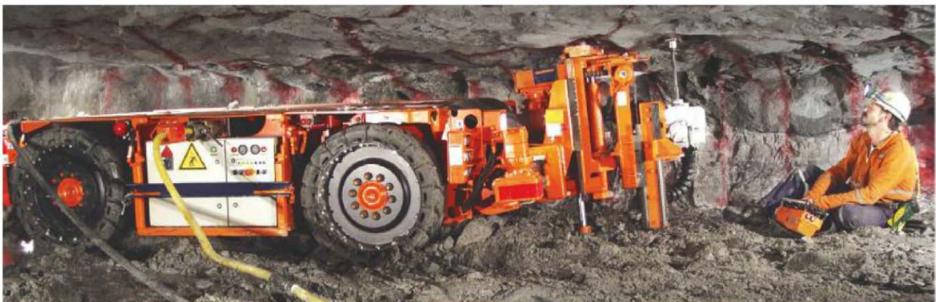
Sandvik designed the skid-steer DS110L bolting rig for operation in stope heights as low as 1.1 m.
