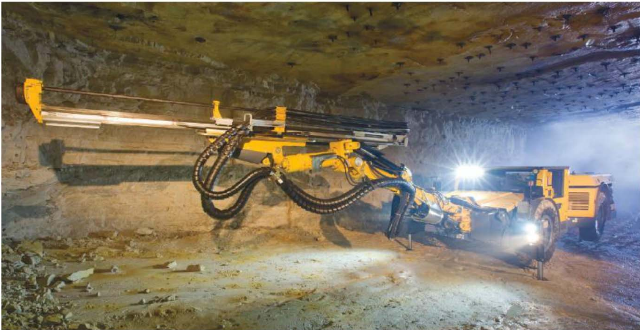
Introduced in 2011, Atlas Copco's Boomer M1 L drill rig is designed for use in low- to-medium-height operations. Its articulated carrier simplifies tramping in narrow headings.
