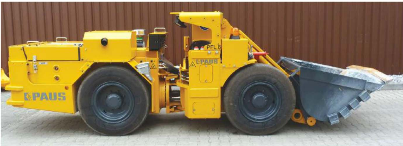
While the PFL 8 is one of the smallest LHDs available today, it is built to withstand the rigors of narrow-vein operations.
